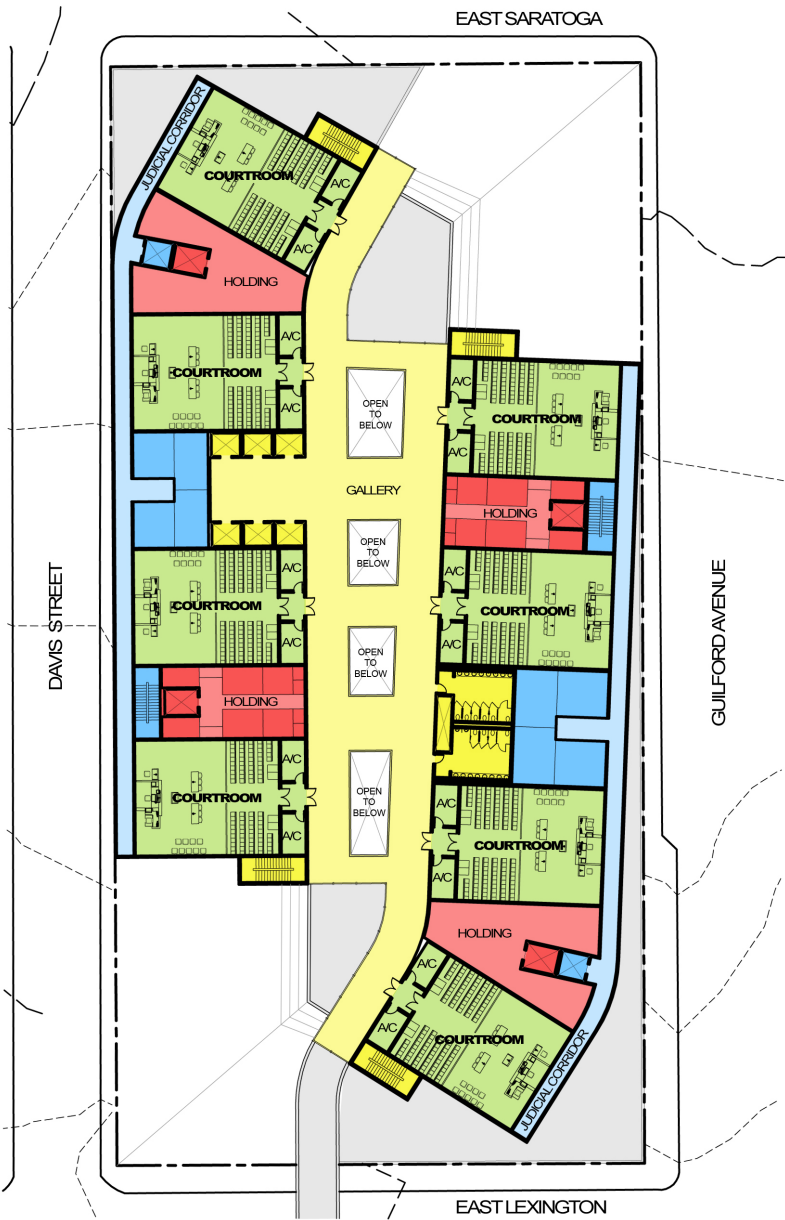
Figure 8-12 Option C: North Site—Proposal for 8 courtrooms per floor: typical courtroom floor plan.
